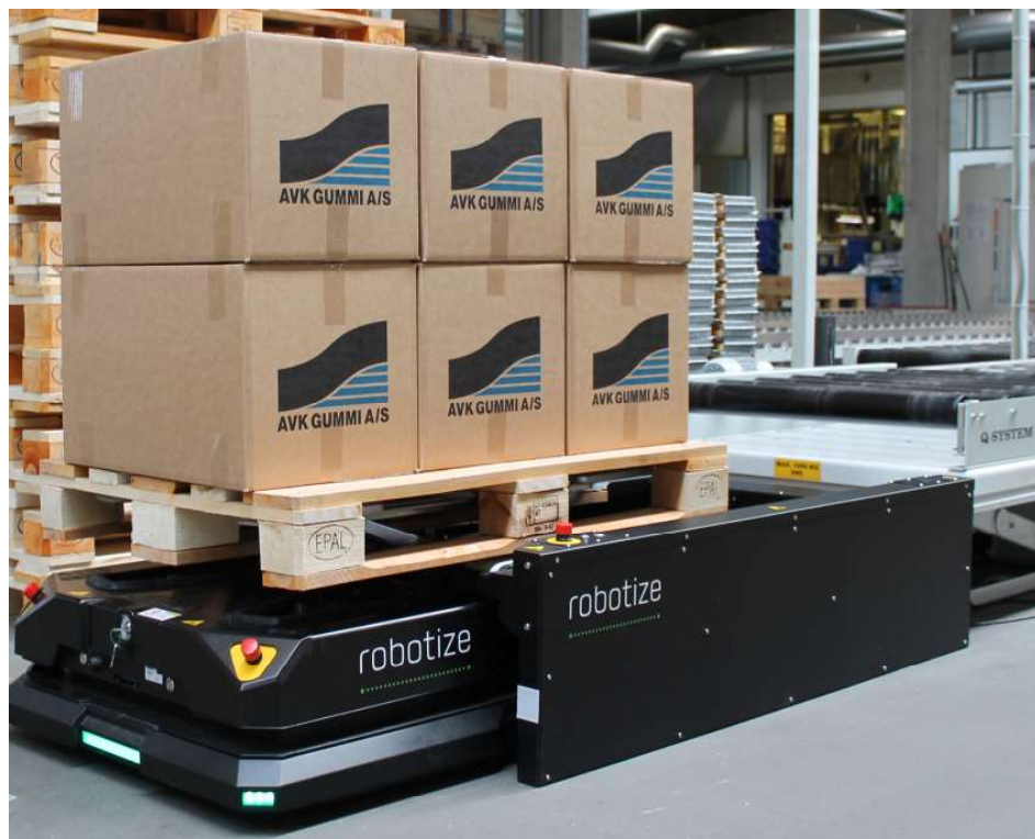
Robotize transports tools from the tooling department to the machines and finished goods from the production area to the shipping department.
